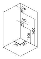
120V 40 amp GFI breaker  $^{1/2^{\prime\prime}}$  MIP for hot and cold water lines 2" drain
